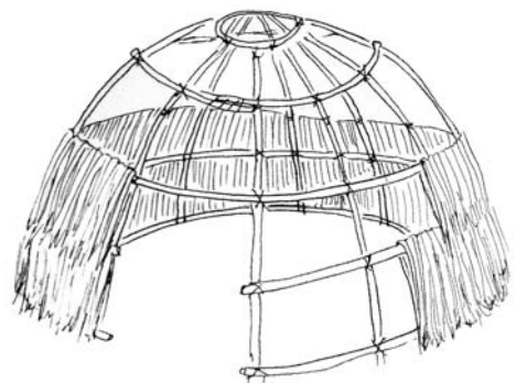
View of the dome-style frame
